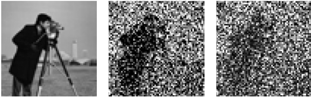
Figure 2.2: We visualize the effect that noisy measurements have on the quality of the spectral estimate when preprocessing functions are not used. On the far left is the original image. In the middle is the spectral estimate when there is no noise added to the phaseless measurements. In the last column is the spectral estimate when additive white Gaussian noise with variance \sigma^2 = 5 is added to each phaseless measurement.
