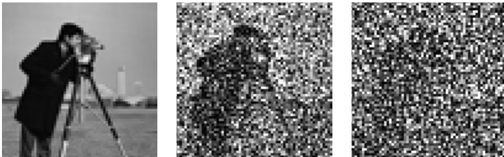
Figure 2.4: We visualize the effect of using the wrong preprocessing function. On the far left is the original image. In the middle is the spectral estimate when the optimal preprocessing function, \mathcal{T}_5(\cdot) , is used, while the last column is the spectral estimate when incorrect preprocessing function, \mathcal{T}_1(\cdot) , is used.
