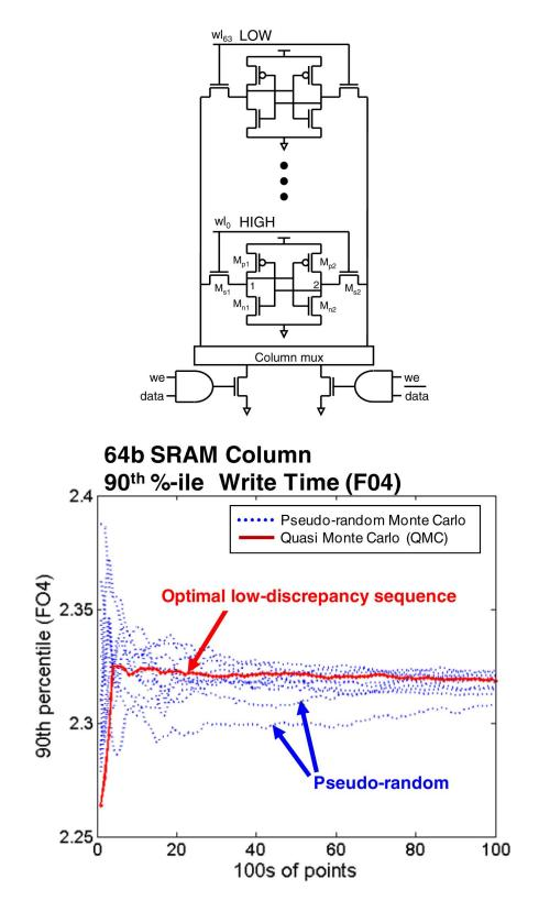
Fig. 12. Computing ninetieth percentile write-time for a full 64-bit SRAM column (top), 90 nm CMO5, across statistical process variation, using QMC methods from [136]. The circuit has more than 400 statistical variables; the plot shows progress towards convergence for ten random Monte Carlo runs (blue) and one optimal, low-discrepancy QMC run (red). Using the QMC sampling, we converge to the correct answer roughly 10x faster than conventional Monte Carlo sampling.
