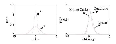
Fig. 13. The quadratic MAX(•) approximation proposed in [1] yields better accuracy than a simple linear approximation.
