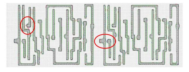
Fig. 8. Lithography simulation showing hotspots as a function of pattern neighborhood.
