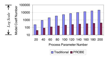
Fig. 11. PROBE [1] significantly reduces the number of model coefficients compared with the traditional full-rank quadratic approximation.
