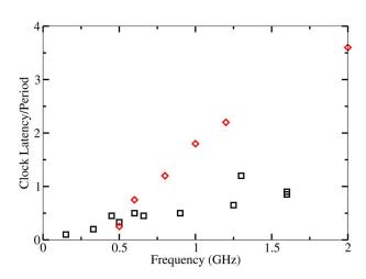
Fig. 2. Global clock latencies from published microprocessor designs; circles are tree-based clocks with active deskewing; squares are tree-driven grid clocks.
