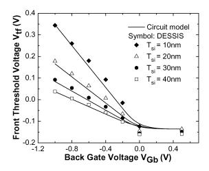
Fig. 5. The coupling between  $V_{\rm Tf}$  and  $V_{\rm Gb}$  in a FinFET device.
