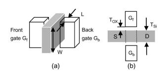
Fig. 4. The structure of a FinFET device: (a) three-dimensional view and (b) the top view of both.
