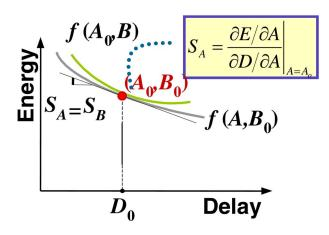
**Fig. 1.** Delay-constrained energy minimization to meet delay constraint *D*<sub>0</sub>. Minimum energy occurs at the point at which the sensitivities *S*<sub>1</sub> are the same for all parameters of interest.
