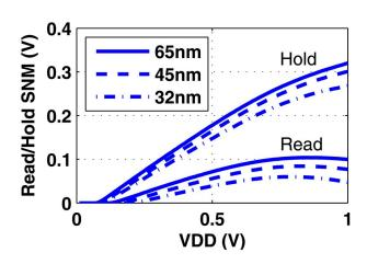
**Fig. 7.** Read SNM versus  $V_{DD}$  using predictive technology models.
