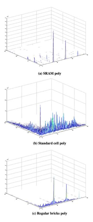
**Fig. 9.** Spatial frequency analysis for (a) SRAM poly, (b) standard cell poly, and (c) regular bricks poly for a 65-nm bulk CMOS process.
