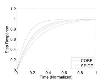
Fig. 10. CORE [1] accurately captures the step response variation of an interconnect network containing 1275 RC elements. Results are plotted at five random Monte Carlo samples.
