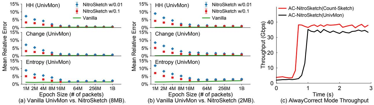
**Figure 11:** (a),(b) Error rates of vanilla UnivMon and NitroSketch with different fixed sampling rates  $p$  (0.1 and 0.01) and memory settings (8MB and 2MB). (c) Throughput over time for AlwaysCorrect NitroSketch with different sketches.
