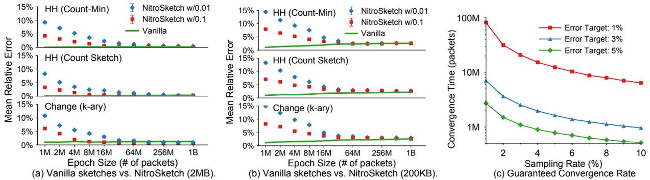
**Figure 12:** (a),(b) Error rates of vanilla sketches and NitroSketch with different fixed sampling rates  $p$  (0.1 and 0.01) and memory settings (2MB and 200KB). (c) Proven convergence time on CAIDA traces.
