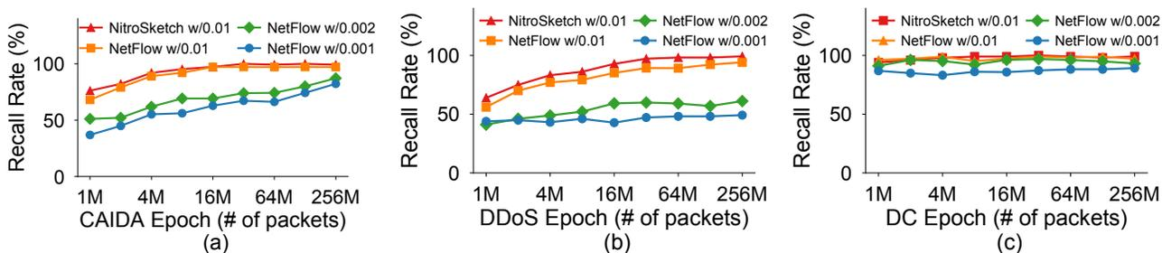
Figure 15: HH recalls of NetFlow with different sampling rates vs. NitroSketch with 0.01, using CAIDA, DDoS, and datacenter traces.
