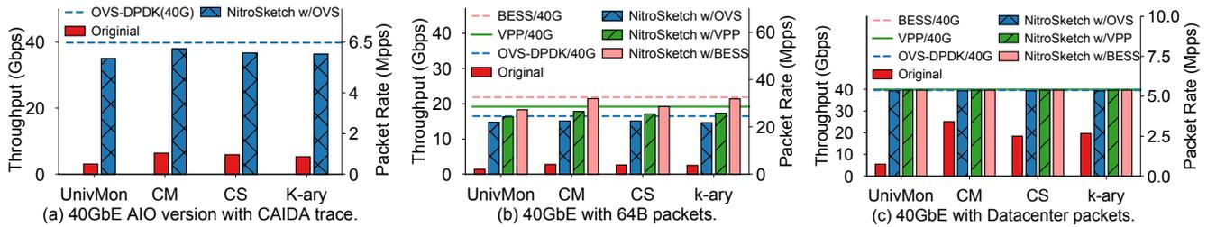
**Figure 8: Throughput (left y-axis) and packet rates (right y-axis) on OVS-DPDK, VPP, and BESS. In (a), OVS-DPDK uses single-thread inline version while in (b) and (c) use a single-thread NitroSketch and another two threads for the switches.**
