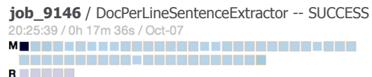
Figure 9: Visual signature of data skew . A node with anomalous task durations (darker color) and high volume of I/O (first nodes in the list) can signal data skew.
