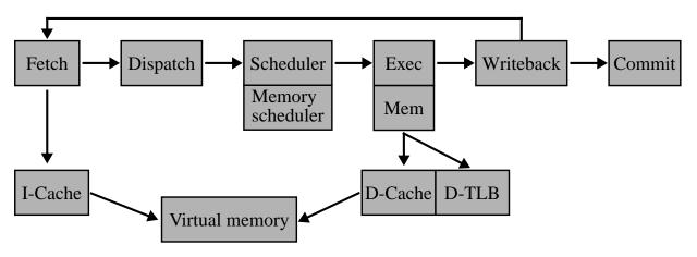
Figure 5. Pipeline for sim-outorder
