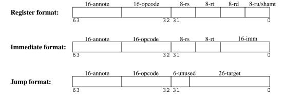
Figure 3. SimpleScalar architecture instruction formats
