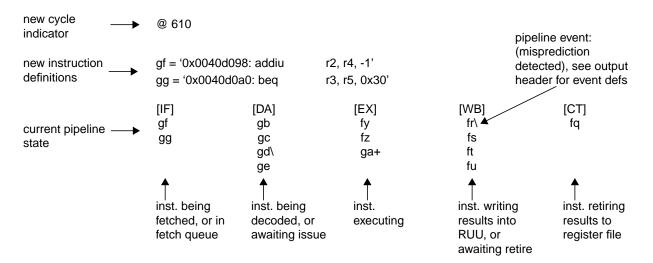
Figure 7. Example of sim-outorder pipetrace
