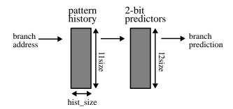
Figure 6. 2-level adaptive predictor structure
