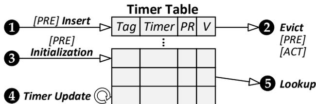
Figure 8: High-level overview of timer table operations.
