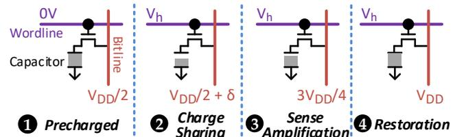
Figure 4: Cell charge levels during DRAM operations.
