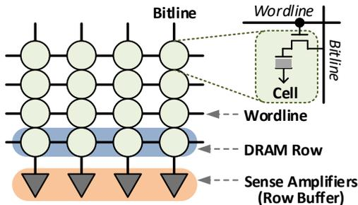
Figure 2: DRAM subarray organization and cell structure.
