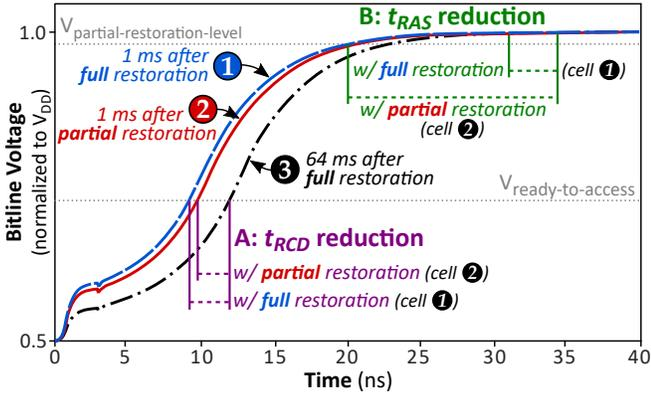
Figure 7: Effect of charge level and restoration level on  $t_{RCD}$  (activation) and  $t_{RAS}$  (restoration) latency reductions.
