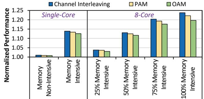
Figure 15: Speedup for different address mapping schemes.
