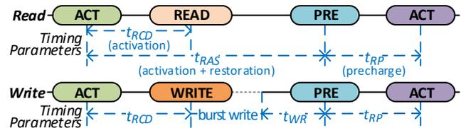
Figure 3: Commands and timing parameters for reading (top) and writing (bottom) data from/to DRAM.
