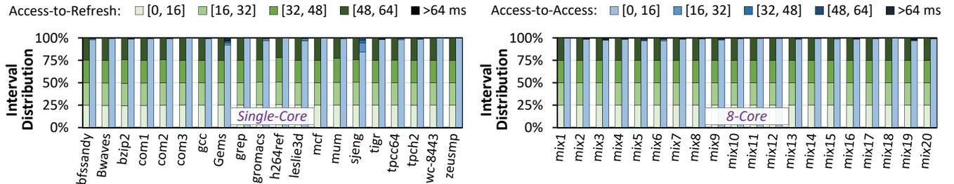
Figure 5: Distribution of access-to-access and access-to-refresh intervals for single-core (left) and 8-core (right) workloads.  $[a, b]$  represents all intervals of length  $t$  where  $a \leq t < b$ , with  $a, b$ , and  $t$  expressed in milliseconds.
