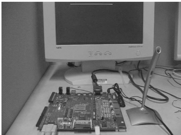
Figure 11. Fully custom hardware speech recognition system setup
