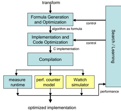
**Fig. 2.** Integrating power simulation into the SPIRAL environment
