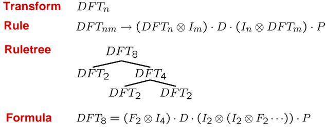
**Fig. 1.** Using rules to decompose a transform into a rule tree and formula.
