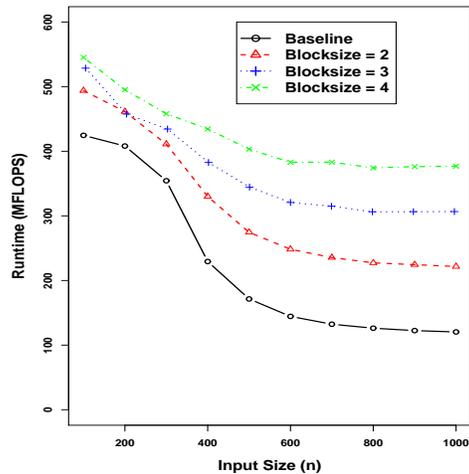
Fig. 2. LU Baseline algorithm plotted against the Blocked algorithm with varying block sizes.
