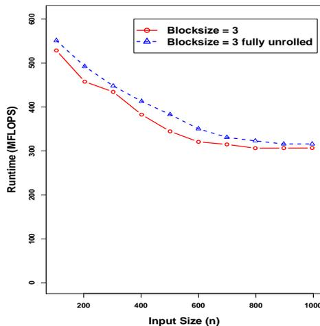
**Fig. 4.** LU blocked algorithm with block size of 3 plotted against a loop unrolled implementation.
