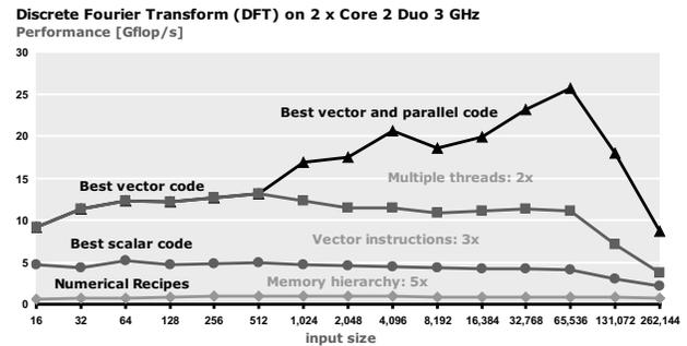
**Fig. 1.** Performance of four single precision implementations of the discrete Fourier transform. The operations count is roughly the same. *The labels in this plot are too small.*
