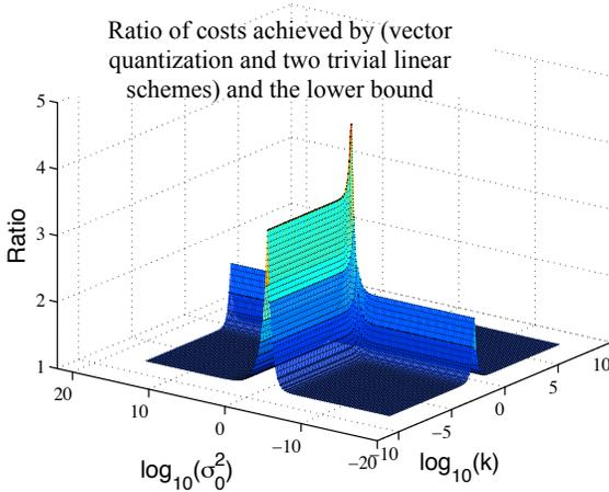
The ratio of our upper bound (obtained by using the **vector quantization strategy** and the two trivial linear schemes) and our lower bound is no greater than 4.45. Analytically, we can show that the ratio is bounded by 11. Observe that the ratio is quite close to 1 for “most” values of  $k$  and  $\sigma_0^2$ .
