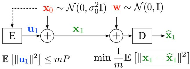
We extend the counterexample to a vector problem of vector length  $m$ . Interpreted as an information theory problem, the first controller is an “encoder” that drives  $\mathbf{x}_0$  to  $\mathbf{x}_1$  using an average power constrained input  $\mathbf{u}_1$ . The second controller, acting as a “decoder”, estimates  $\mathbf{x}_1$ . The objective is to minimize the mean-square error in estimation of  $\mathbf{x}_1$ .
