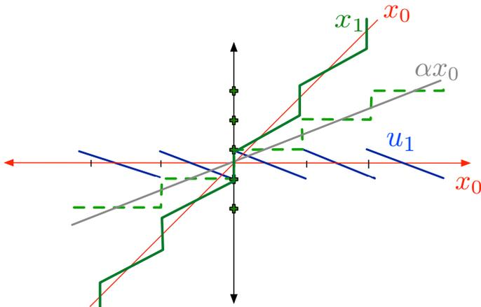
The quantization to intervals strategies in [Baglietto et al][Lee, Lau, Ho] can be thought of as follows. First, the state  $x_0$  is scaled down to a shadow state  $\alpha x_0$ . This shadow state is now quantized, and the resulting  $u_1$  is applied to  $x_0$ .
