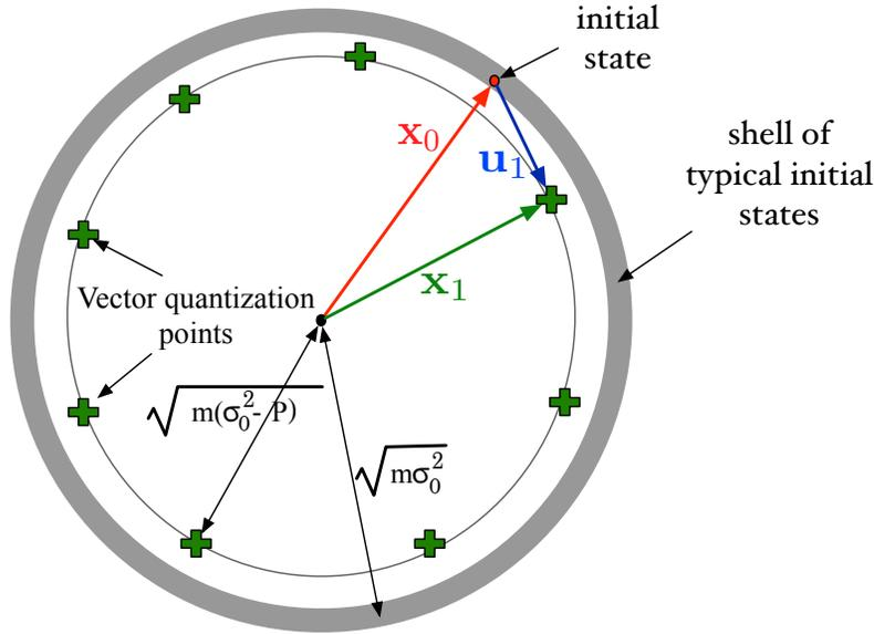
Our first nonlinear strategy is a vector quantization based strategy where *the first controller drives the state  $\mathbf{x}_0$  to the nearest quantization point*. These quantization points have power smaller than  $\sigma_0^2$ . Provided the number of quantization points is sufficiently small, they can be decoded correctly at the second controller. Asymptotic cost is  $k^2 \sigma_w^2$  and 0 for the first and the second stage respectively.
