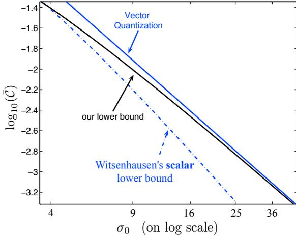
Witsenhausen's lower bounding technique does not extend to the vector case. We provide the following **new lower bound** to the optimal costs which is valid for all vector lengths  $m \geq 1$ ,
