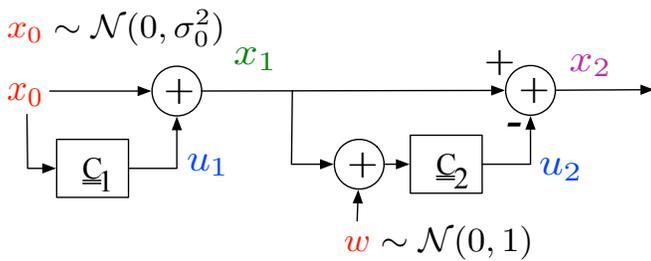
In the first stage,  $\underline{C}_1$ , the first controller, acts on the initial state  $x_0$  using its input  $u_1$  and forces it to  $x_1$ . In the second stage,  $\underline{C}_2$ , the second controller observes  $x_1 + w$  and acts on  $x_1$  to obtain state  $x_2$ . The first stage cost is  $k^2 u_1^2$  and the second stage cost is  $x_2^2$ . Thus, the total cost is  $\mathcal{C} = k^2 u_1^2 + x_2^2$ .
