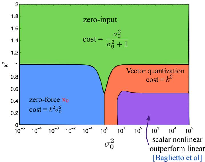
In the zero-forcing linear strategy, *the first controller chooses  $\mathbf{u} = -\mathbf{x}_0$ , and thus  $\mathbf{x}_1 = 0$* . In the zero-input linear strategy, *the first controller uses  $\mathbf{u} = 0$ , and the second controller estimates  $\mathbf{x}_1$  based on its observation*.
