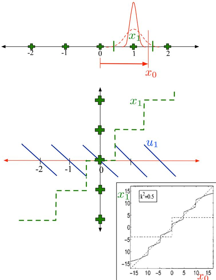
The counterexample contains an **implicit communication channel**. Using quantization-based signaling strategies, it was shown in [Mitter and Sahai, 99] that the ratio of cost attained by the optimal linear strategy to that attained by the optimal nonlinear strategy can be arbitrarily large.
