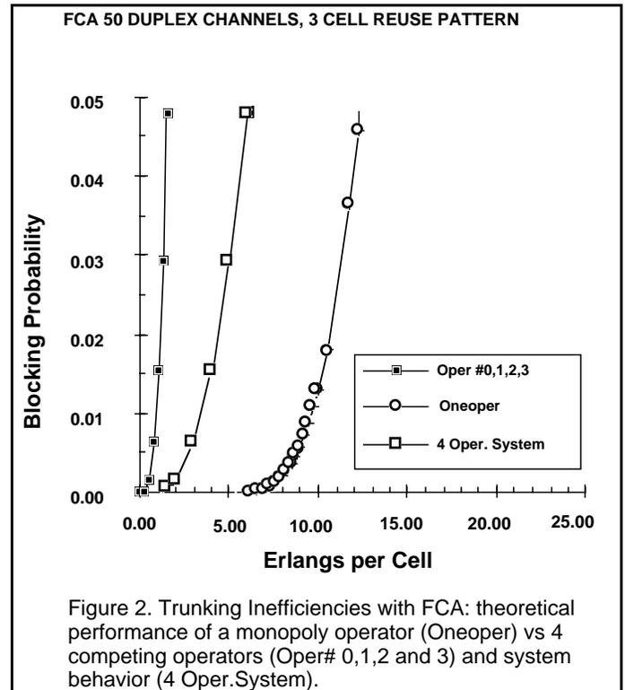
Figure 2. Trunking Inefficiencies with FCA: theoretical performance of a monopoly operator (Oneoper) vs 4 competing operators (Oper# 0,1,2 and 3) and system behavior (4 Oper.System).
