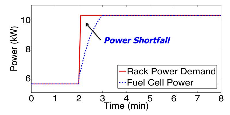
Can lead to server damage or shut down
