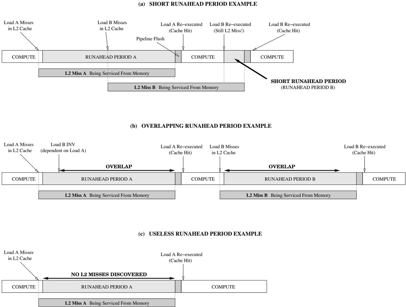
Figure 3. Example execution timelines illustrating the causes of inefficiency in runahead execution (short, overlapping, useless runahead periods) and how they may occur.
