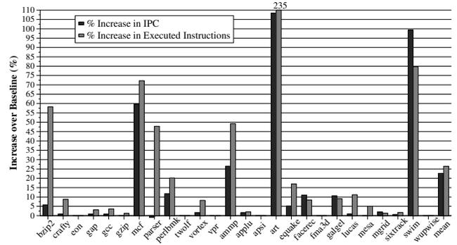
Figure 2. Increase in IPC performance and executed instructions due to runahead execution.
