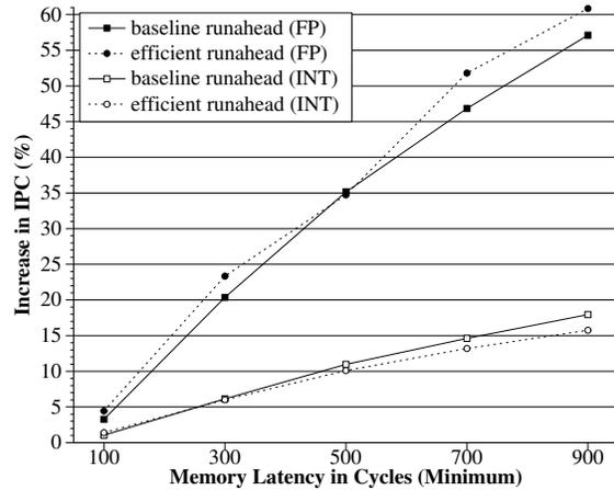
Figure 5. Extra instructions and IPC increase with and without the efficiency techniques for five different memory latencies. Data shown are averaged separately over integer (INT) and floating-point (FP) benchmarks.
