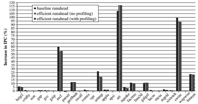
Figure 4. Increase in executed instructions and IPC due to runahead execution after incorporating all the efficiency techniques.
