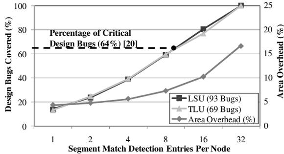
Figure 16. Area overhead versus design bug coverage
