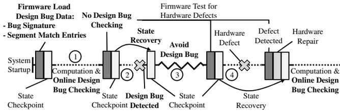
Figure 15. Unifying design bug detection and defect detection
