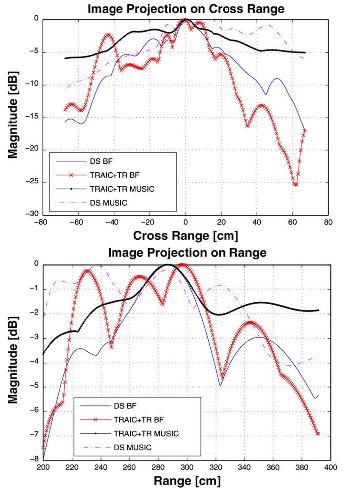
Fig. 3. The projection onto cross range and range for the images in Fig. 2. Top—Cross range; Bottom—Range. TRAIIC shows a narrower main lobe, deeper null, and lower sidelobes relative to DS imaging.
