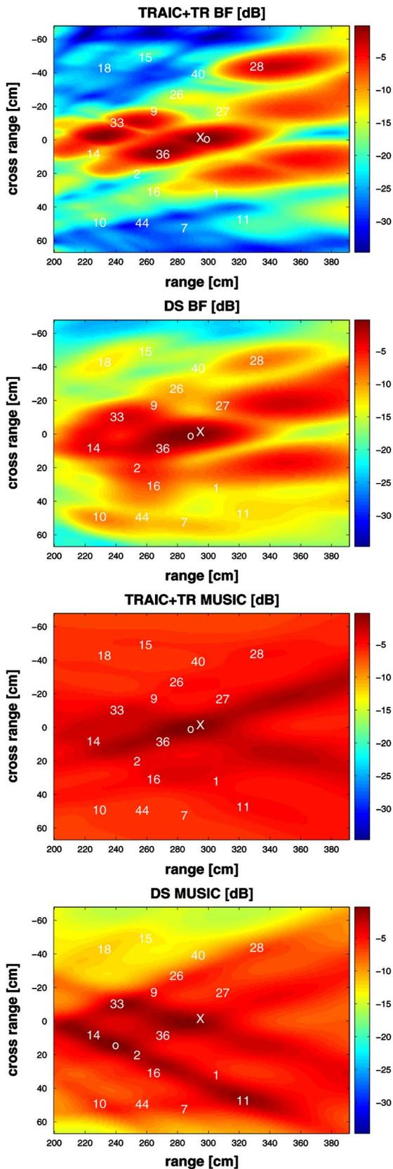
Fig. 2. Time Reversal imaging with 17 scatterers and 1 target. Numbers indicate locations of the scatterers,  $\times$  and  $\circ$  indicate the exact location of the target and the peak value of the image, respectively. Uppermost—TRAIIC+TRBF. Middle—DSBF. Lower—TRAIIC+TR MUSIC. Lowest—DS MUSIC. All images are plotted within the same range ( $0 \sim -34$  dB).
