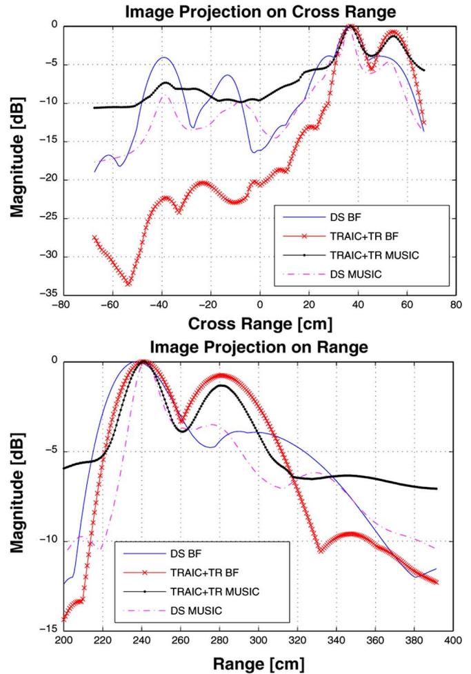
Fig. 5. The projection onto cross range and range for the formed image in Fig. 4. Top—Cross range projection. Bottom—Range projection. TRAIC+TRBF yields two lobes corresponding to two target locations.
