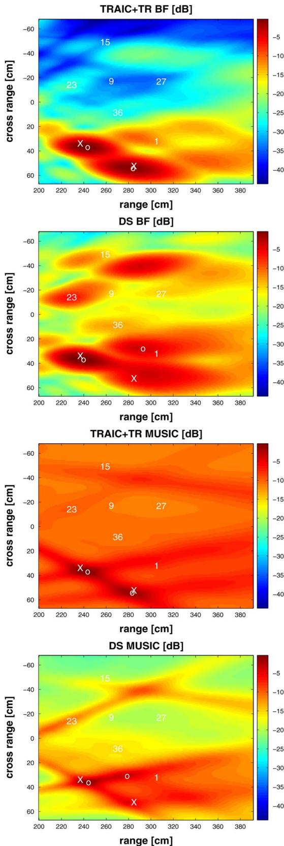
Fig. 4. Time Reversal imaging with 6 scatterers and 2 targets. Numbers indicate locations of the scatterers,  $\times$  and  $\circ$  indicate the exact location of the target and the peak value of the image, respectively. Uppermost—TRAIC+TR beamforming. Middle—DSBF. Lower—TRAIC+TR MUSIC. Lowest—DS MUSIC. All images are plotted within the same range (range 0 ~ -45 dB).
