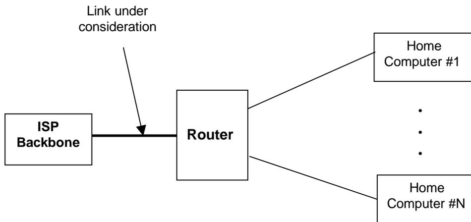
Figure 9: Modem router's link to the ISP backbone
