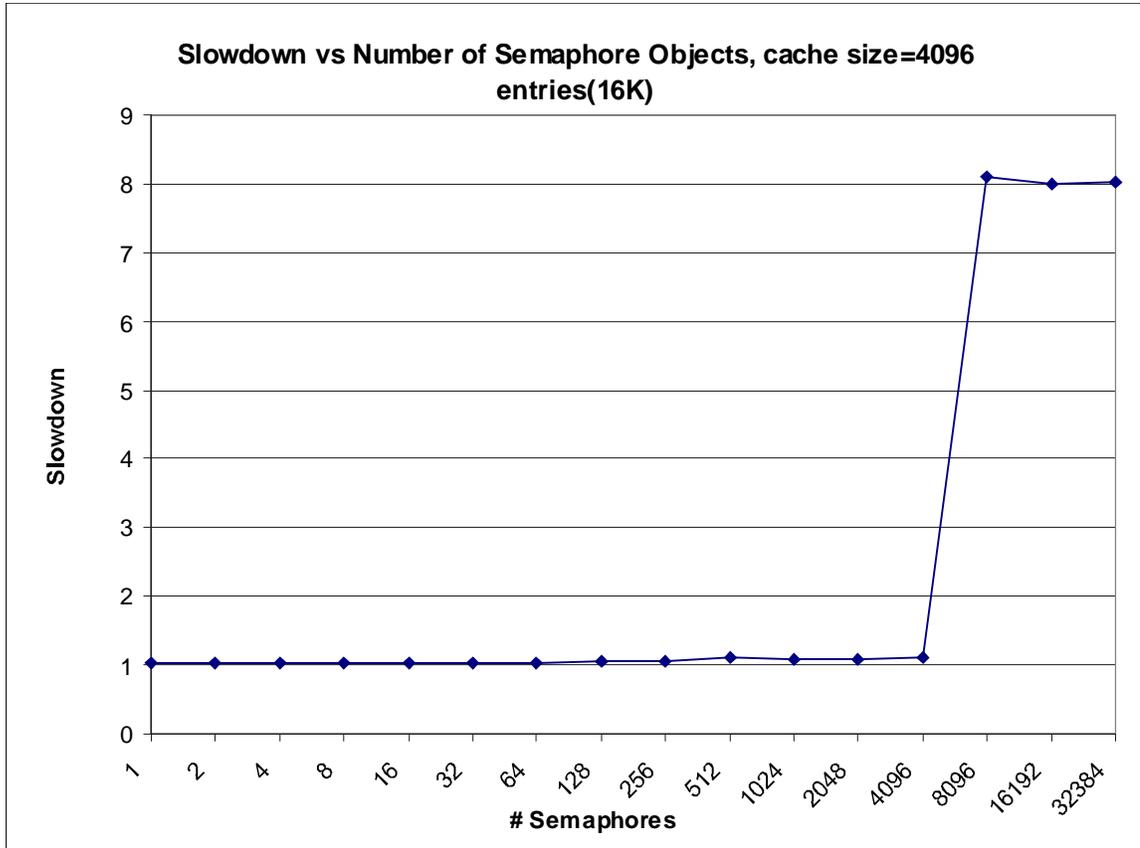
Figure 26. Slowdown of synthetic benchmark using robust process synchronization functions with large cache size
