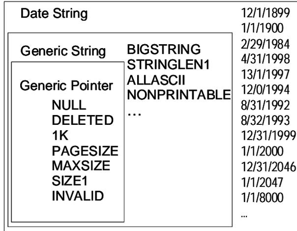
Figure 3. A Date String type inherits tests from Generic String and Generic Pointer
