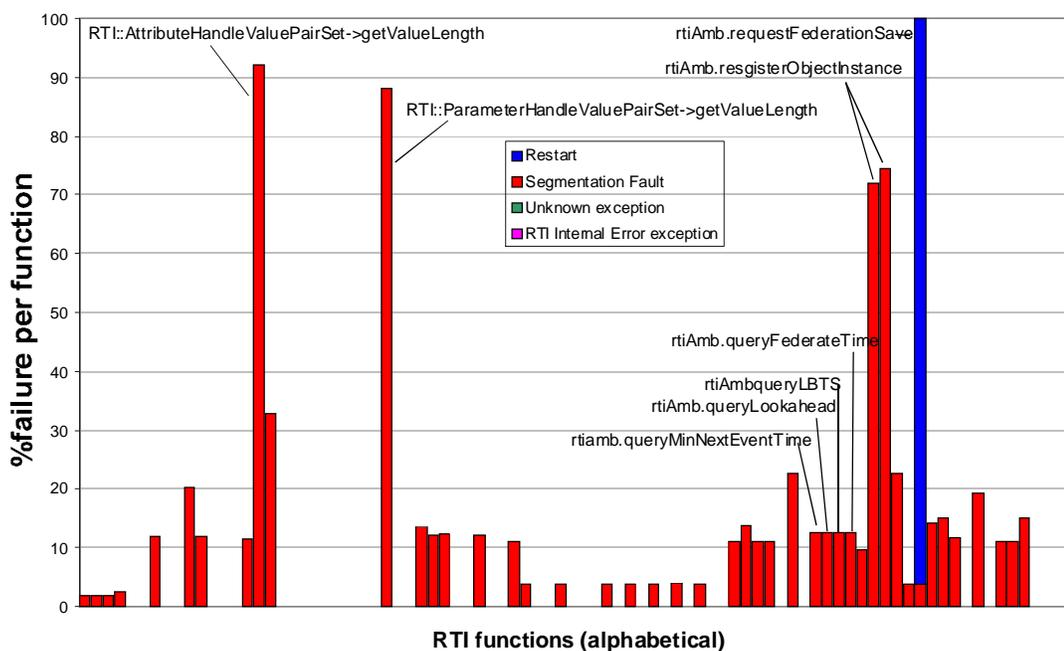
Figure 29. Robustness failure rate for RTI 1.3.5 under SunOS 5.6. Overall Average failure rate = 10.0% from [fernsler99].
