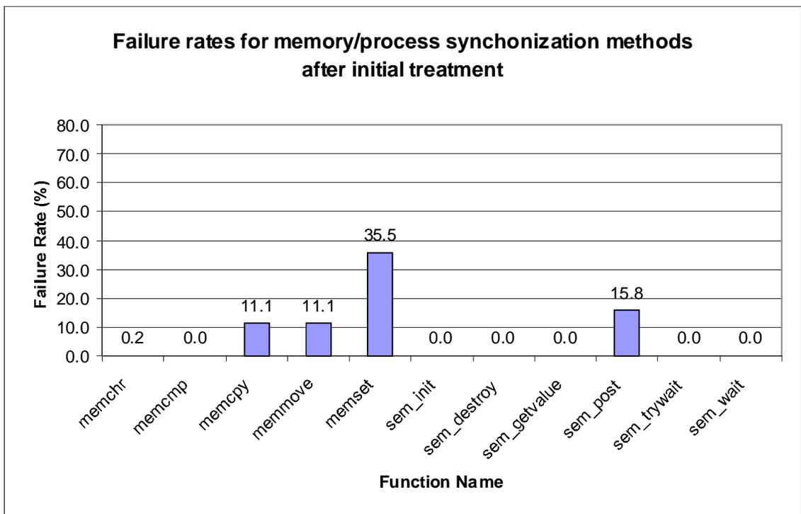
Figure 18. Failure rate of memory and process synchronization functions after initial treatment
