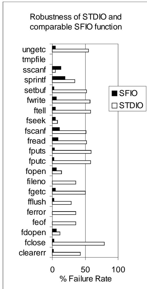
Figure 11. Robustness failure rates for SFIO, STDIO compared for 20 functions with direct functional equivalence as measured on the Linux test system. Failure rates on Digital Unix were lower for some SFIO functions and are addressed later in Section 5.2
