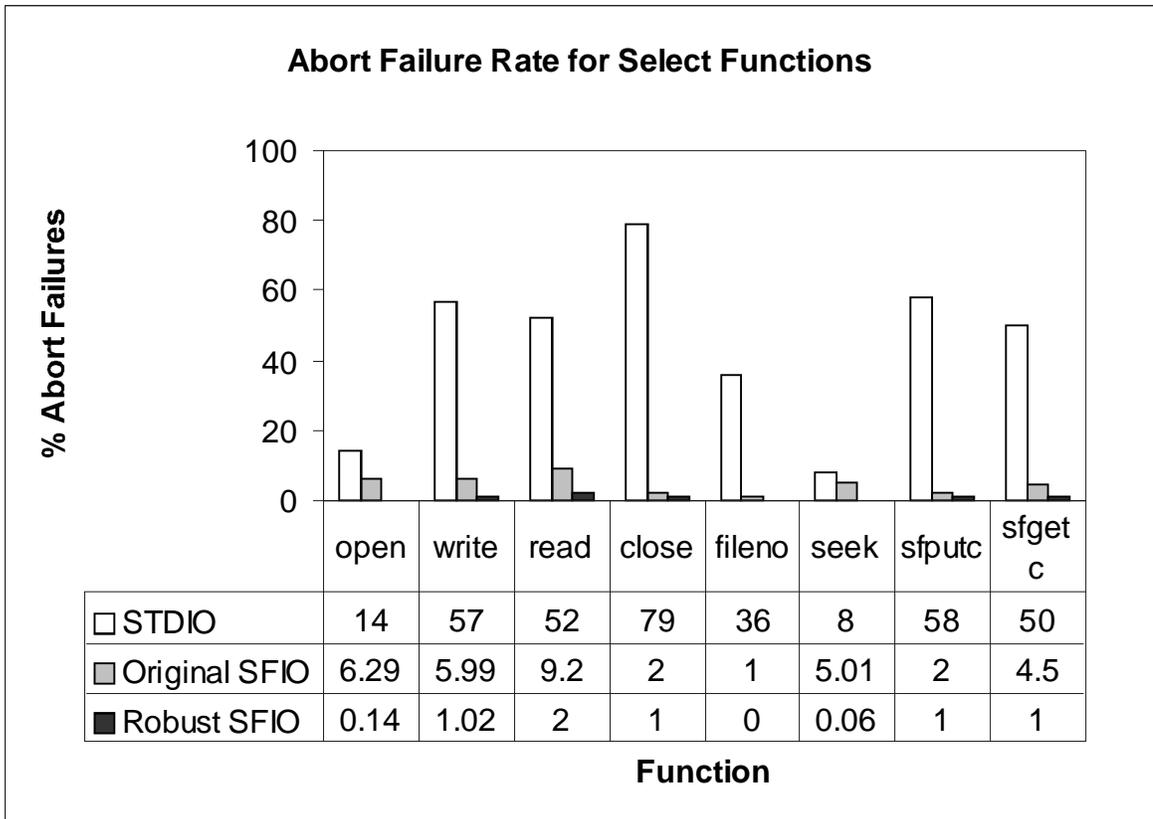
Figure 12. Abort Failure Rate for Select SFIO Functions under Linux
