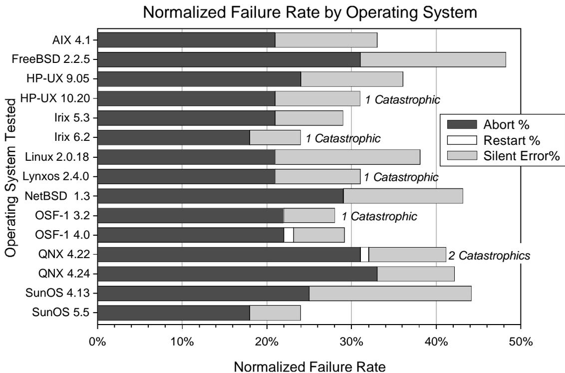
Figure 9. Adjusted, normalized robustness failure rates after using multi-version software techniques. Results are APPROXIMATE due to the use of heuristics.
