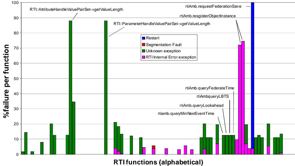
Figure 30. Robustness failure rate for RTI 1.3.5 under Digital Unix 4.0. Overall Average failure rate = 10.1% from [fernsler99].
