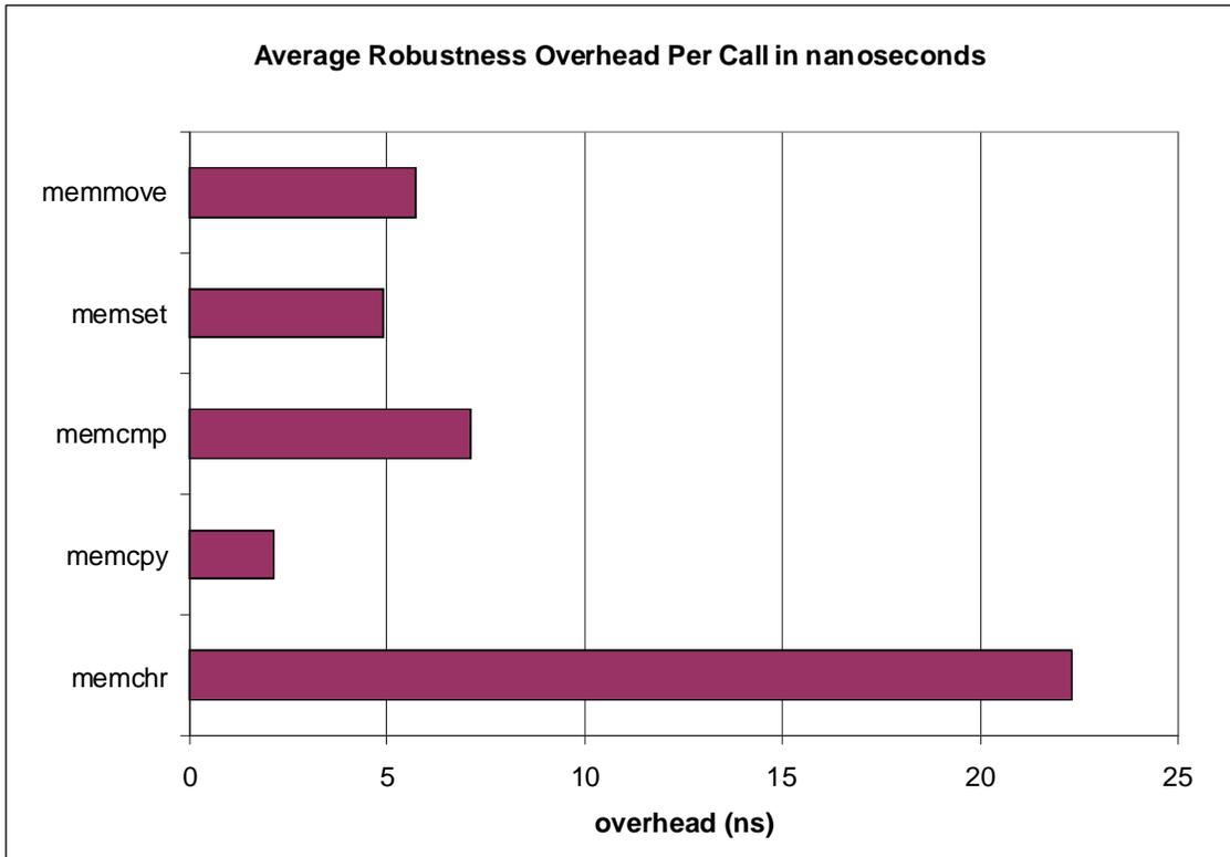
Figure 28. Absolute robustness overhead for memory functions in nanoseconds
