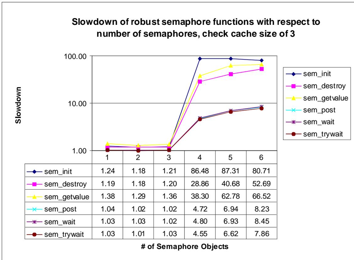
Figure 22. Iterative performance slowdown of robust process synchronization functions
