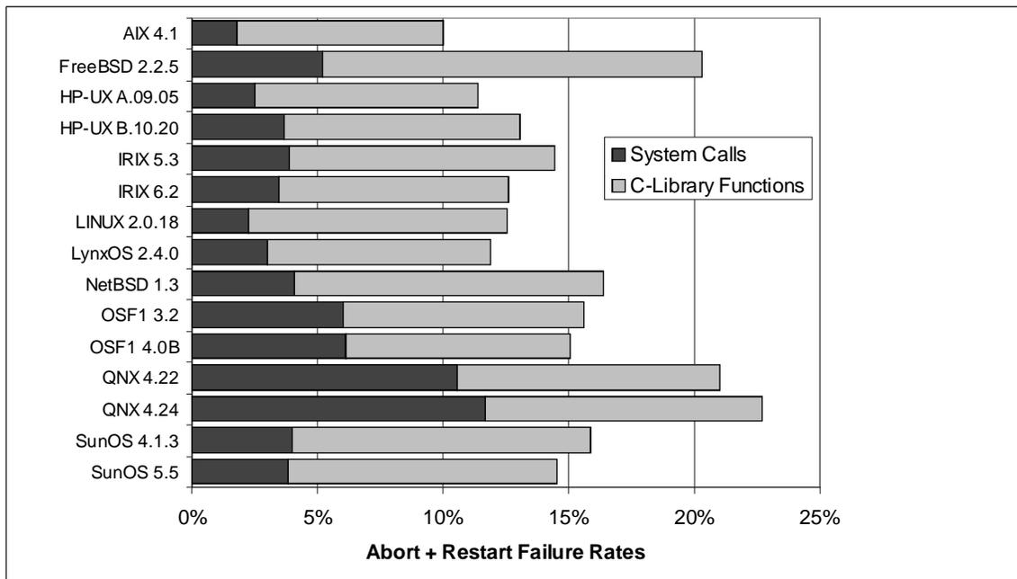
Figure 8. The C-Library functions contribute a large proportion of the overall raw failure rates
