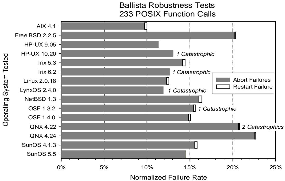
Figure 6. Normalized failure rates for POSIX operating systems
