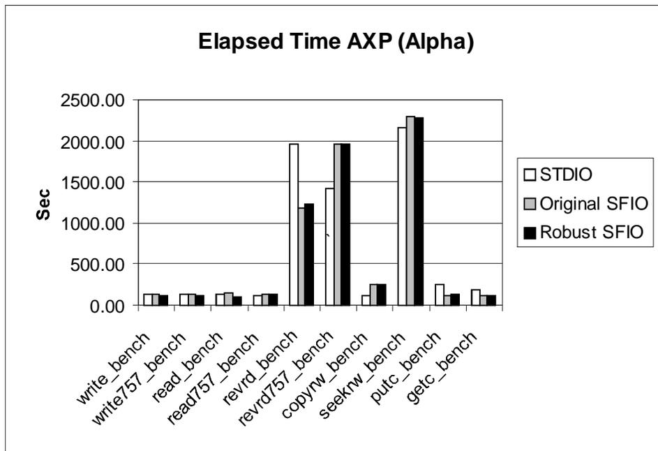
Figure 14. Elapsed time of benchmark running on the AXP (Alpha) architecture
