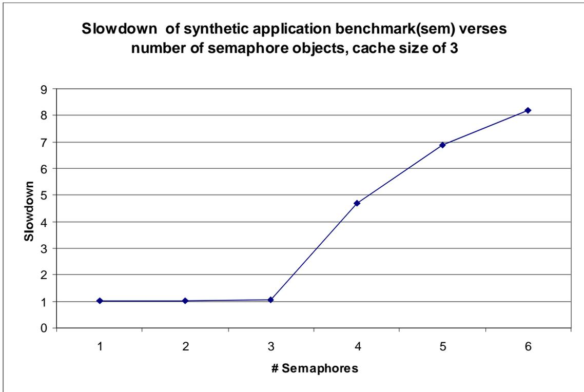
Figure 25. Slowdown of synthetic benchmark using robust process synchronization functions
