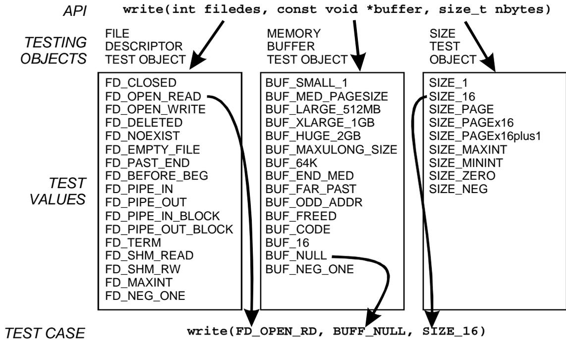
Figure 5. Ballista test case generation for the `write()` function. The arrows show a single test case being generated from three particular test values; in general, all combinations of test values are tried in the course of testing.
