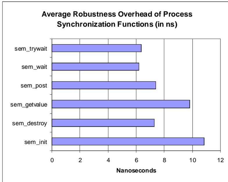
Figure 27. Absolute robustness overhead for process synchronization functions in nanoseconds
