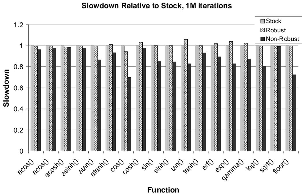
Figure 10. Performance of libm variants normalized to the unmodified source.
