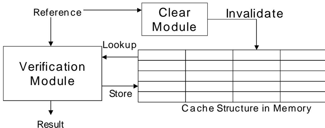
Figure 21. The software implemented robustness check cache
