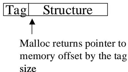
Figure 19. Altered malloc helps address fundamental robustness limitation
