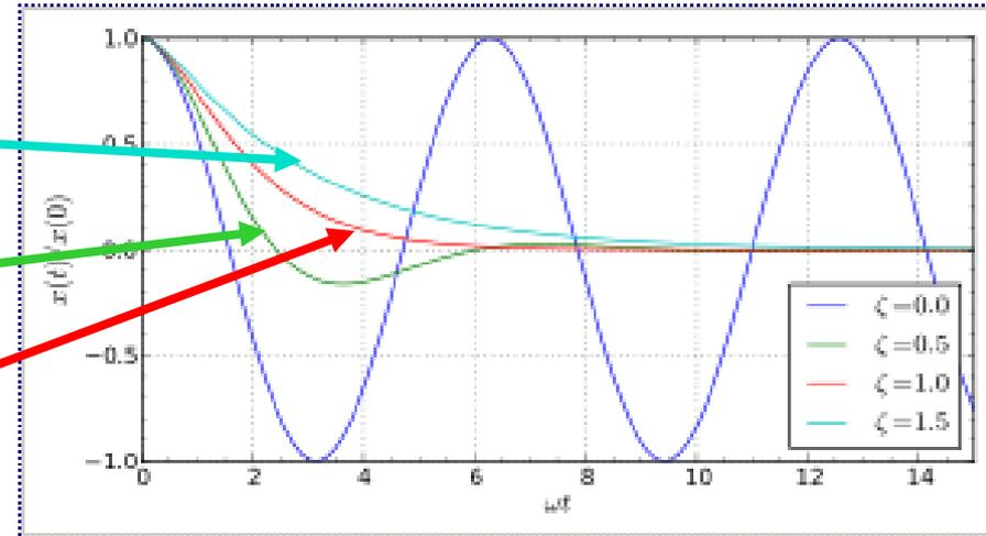
Time dependence of the system behavior on the value of the damping ratio  $\zeta$ , for undamped (*blue*), under-damped (*green*), critically damped (*red*), and over-damped (*cyan*) cases, for zero-velocity initial condition.
