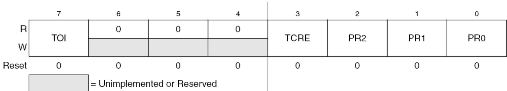
Figure 15-19. Timer System Control Register 2 (TSCR2)
