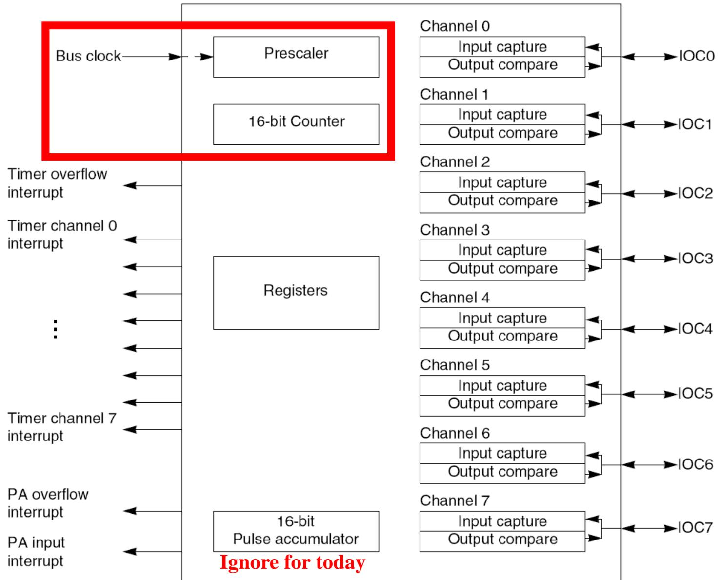
Figure 15-1. TIM16B8CV1 Block Diagram
