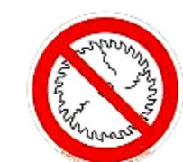
6110 -ISO Do Not Operate With Damaged Blade
