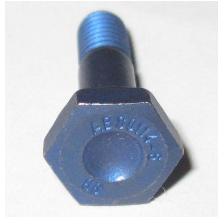
Airbus A-380 bolt with part tracking information.
