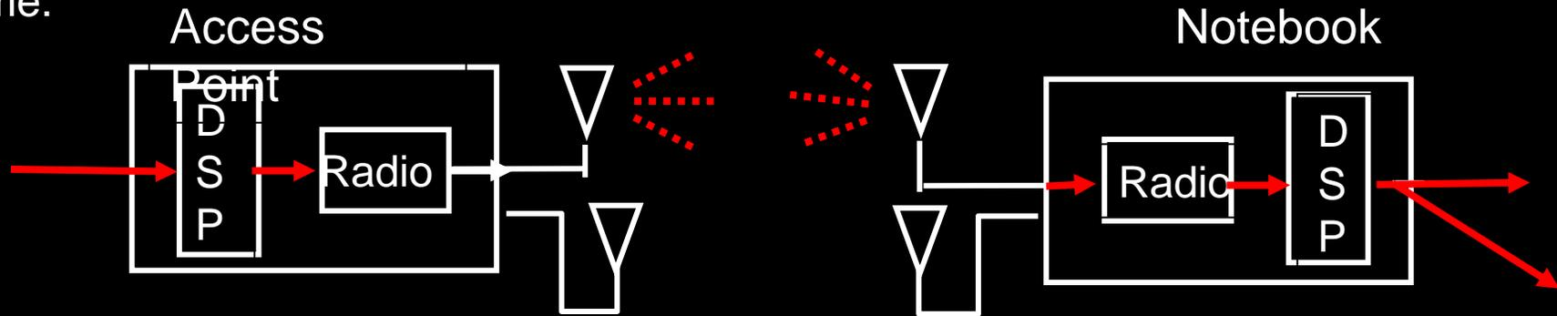
MIMO use multiple radios and multiple antennas at the same time.
