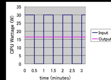
Thermal Capacitor can temporarily store heat
