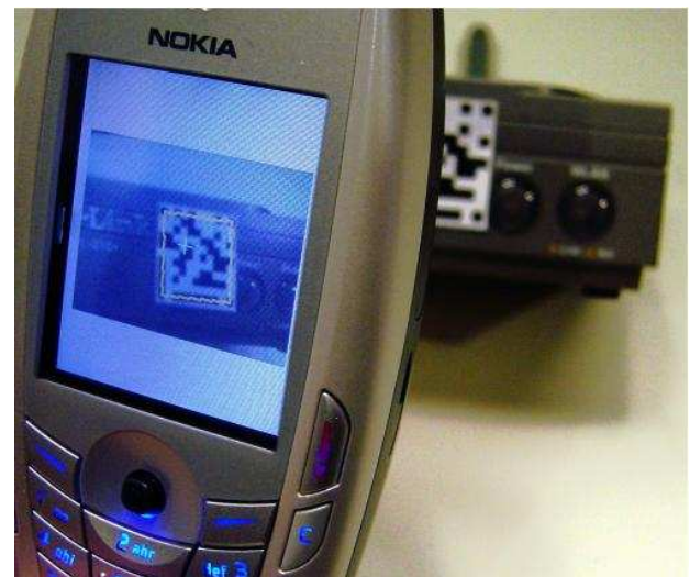
Figure 3. Phone running SiB scanning a barcode on an 802.11 access point.
