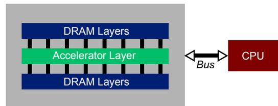
Fig. 2: 3D-stacked offload accelerator.
