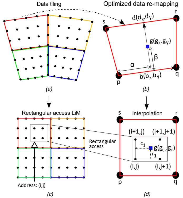
Fig. 4: Data re-mapping through basis vector transform for each grid block.
