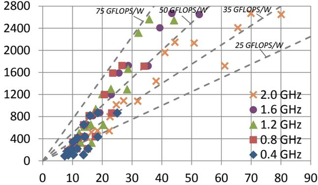
Fig. 9: Design space exploration for performance and power evaluation.
