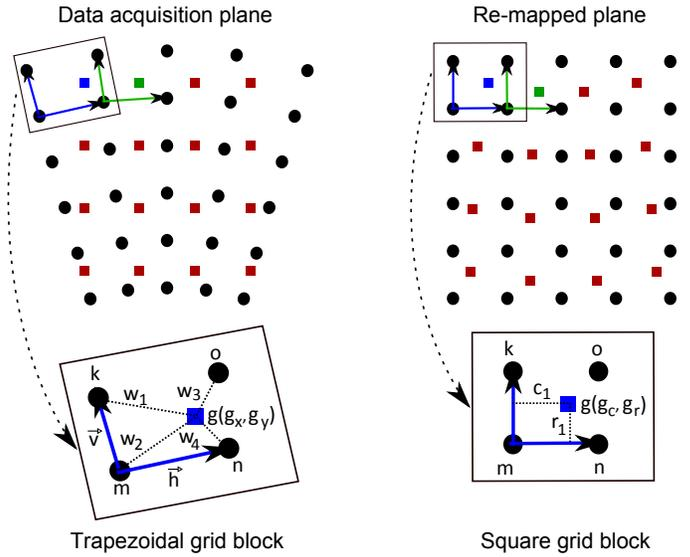
Fig. 3: Data re-mapping through basis vector transform for each grid block.
