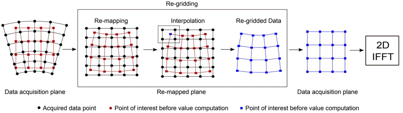
Fig. 1: Different stages of SAR image reconstruction algorithm.
