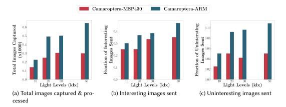
Fig. 11. Figures (a) to (c) show the performance of Camaroptera with our MSP-based design, and using an ARM Cortex-M4 board to run the DNN. While using an ARM core to replace the MSP430 enables Camaroptera to perform better, the lack of FRAM support in commercial ARM cores justifies our choice of building Camaroptera around an MSP430 MCU.
