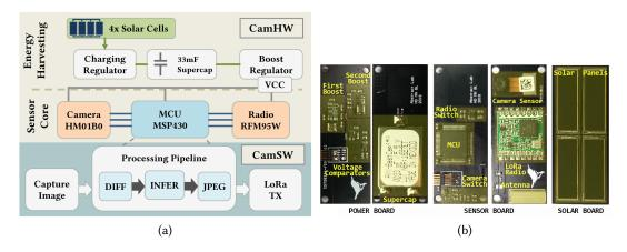
Fig. 3. (a) System overview of Camaroptera. (b) Camaroptera prototype PCBs.
