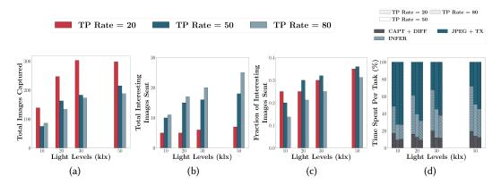
Fig. 8. Figures (a) to (d) show the performance of Camaroptera under different True Positive (TP) rates at different light levels. Here, Camaroptera operates in the *Local Inference* mode with a classifer that has a 10:10 False Positive: False Negative ratio. Changing the TP rate represents different amount of interesting events in the environment.
