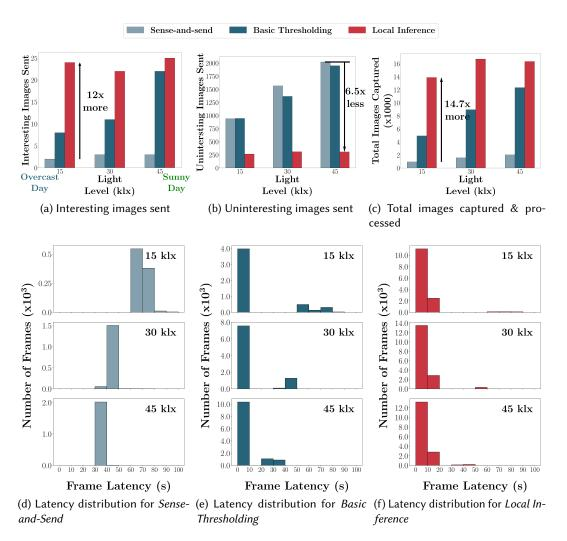
Fig. 7. (a) to (c) show the results of a multi-week experiment demonstrating that the *Local Inference* mode outperforms the *Sense-and-Send* and *Basic Thresholding* modes on Camaroptera, in terms of Interesting images sent, Uninteresting images sent and Total images captured respectively. (d) to (f) show the per-frame latency distribution across the three operating modes, for three different light levels.
