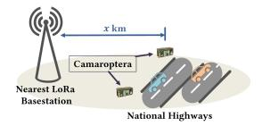
Fig. 1. (a) Camaroptera prototype. (b) Example remote sensing application (national highways), where each device is located far (kms) away from the nearest supporting infrastructure (basestation).
