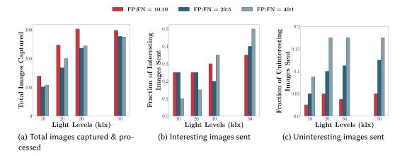
Fig. 9. Figures (a) to (c) show the performance of Camaroptera with different classifiers at different light levels, operating in the *Local Inference* mode. The different classifiers are represented by their False Positive : False Negative (FP:FN) ratio. Here, the True Positive rate for the environment is set to be 20%. Different classifier FP:FN ratios represent different design points for Camaroptera.
