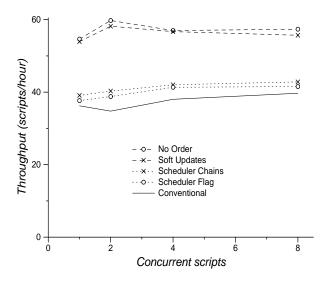
Figure 6: Scheme comparison using Sdet. Each data point is an average of 3 independent executions and all coefficients of variation are less than 0.02. Allocation initialization is enforced only for *Soft Updates*.
