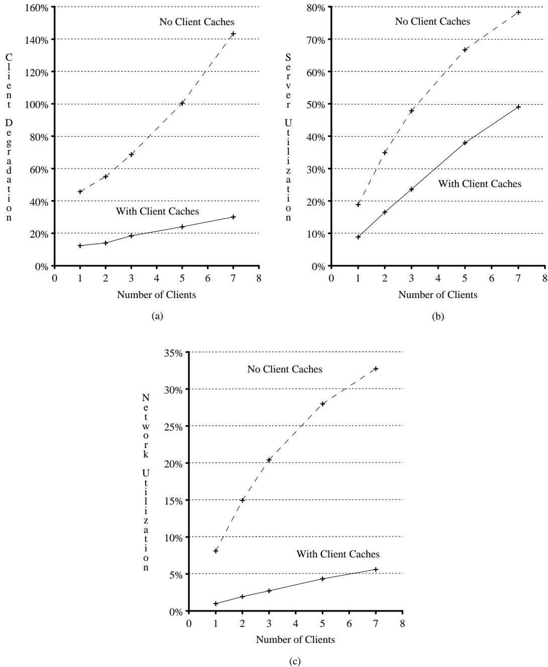
**Figure 4.** Effect of multiple diskless clients running the Andrew benchmark simultaneously on different files in a Sun-3 configuration with variable-size client caches. (a) shows additional time required by each diskless client to complete the benchmark, relative to a single client running with local disk. (b) shows server CPU utilization. (c) shows percent network utilization.
