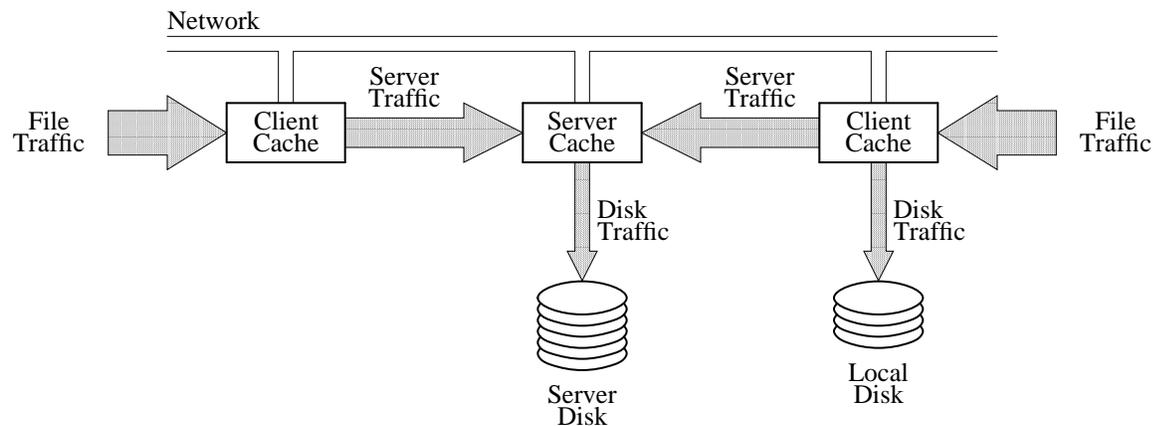
**Figure 1.** File caches in the Sprite system. When a process makes a file access, it is presented first to the cache of the process's workstation ("file traffic"). If not satisfied there, the request is passed either to the local disk, if the file is stored there ("disk traffic"), or to the server where the file is stored ("server traffic"). Servers also maintain caches in order to reduce their disk traffic.
