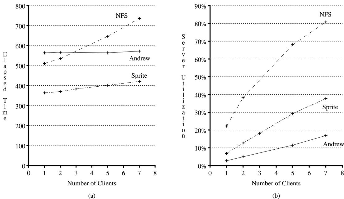
**Figure 5.** Performance of the Andrew benchmark on three different file systems; Sprite, Andrew, and NFS. (a) shows the absolute running time of the benchmark as a function of the number of clients executing the benchmark simultaneously, and (b) shows the server CPU utilization as a function of number of clients. The Andrew and NFS numbers were taken from [HOWA87] and are based Sun-3/50 clients. The Sprite numbers were taken from Table 6 and Figure 4 and re-normalized for Sun-3/50 clients.
