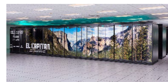
El Capitan 2.8 Eflop/s, 30MW 43k 24-core CPUs + 43k GPUs #1 in Top500
