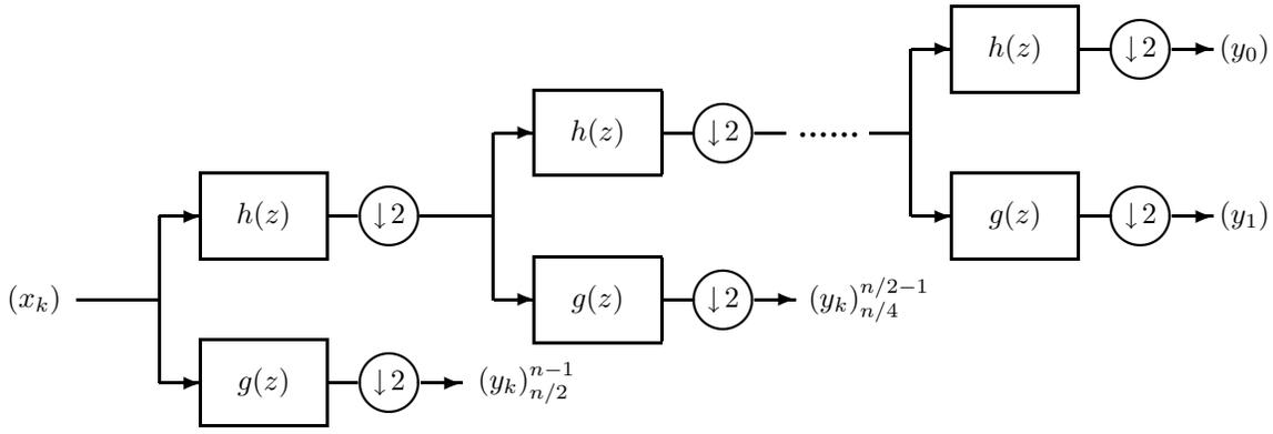
Fig. 2. Filter bank interpretation of the DWT.
