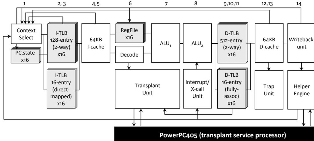
Figure 7 The BlueSPARC engine: a 14-stage instruction-interleaved pipeline
