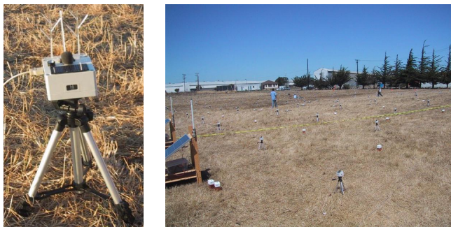
Fig. 5. Hardware for the sensor nodes. (left) Trio sensor node on a tripod. On top is the microphone, buzzer, solar panel, and user and reset buttons. On the sides are the windows for the passive infrared sensors. (right) A live picture from the experiment.
