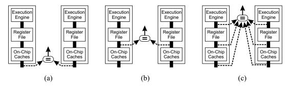
Figure 2: Error detection mechanisms: (a) chip-external, (b) L1 cache interface, (c) full state. Fingerprinting (not shown) provides detection capabilities equivalent to full state comparison, (c).
