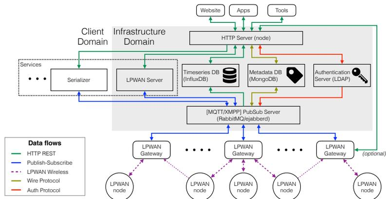
Fig. 1. System architecture for the OpenChirp network
