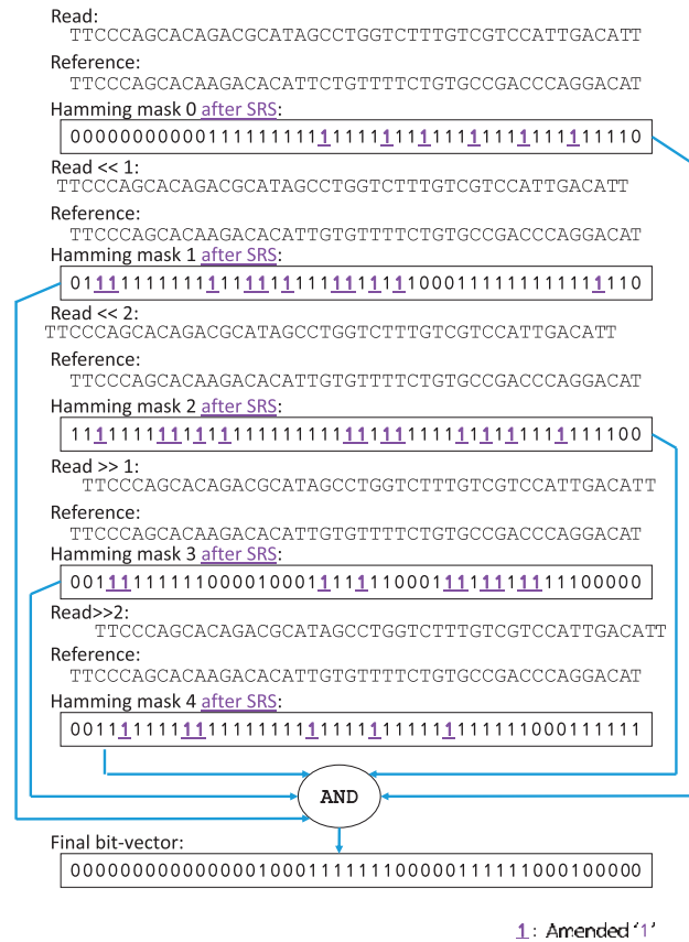
Fig. 3. The incorrect mapping from Figure 2 is filtered correctly by SRS, since most of its short streaks of '0's are turned into amended '1's. Amended '1's are transparent during the AND operations
