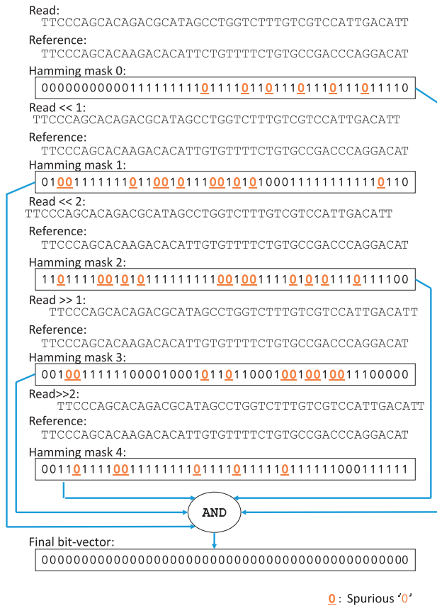
Fig. 2. An example of an incorrect mapping that passes SHM. In this example, during the bit-wise AND operations, short streaks of '0's at different locations in the Hamming masks overwrite (mask out) any '1's in other Hamming mask that are at the same locations. As a result, the final bit-vector of SHM is full of '0's. With SRS, streaks of '0's that are shorter than three are marked as spurious and are subjected to removal later on
