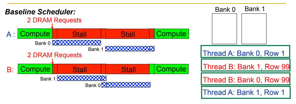
Bank access latencies of each thread serialized Each thread stalls for ~TWO bank access latencies
