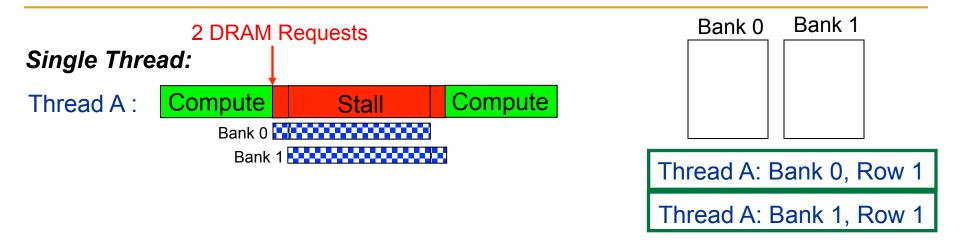
Bank access latencies of the two requests overlapped Thread stalls for ~ONE bank access latency
