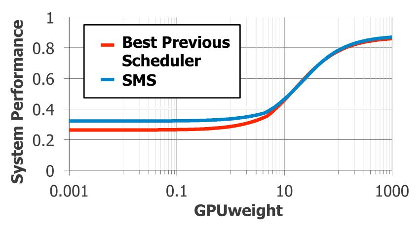
At every GPU weight, SMS outperforms the best previous scheduling algorithm for that weight
