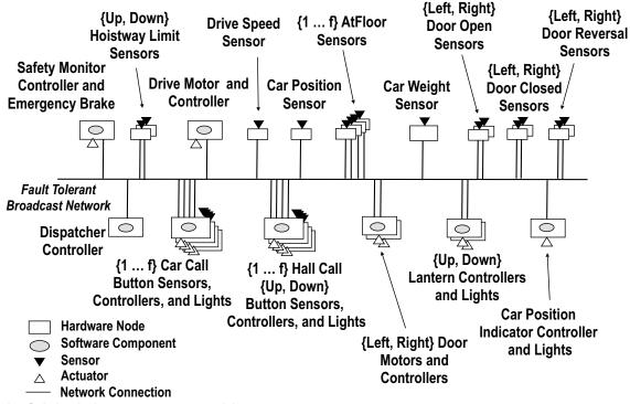
Figure 2. Original elevator system architecture.
