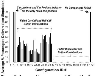
Figure 3. Average % passengers delivered for the original elevator system.
