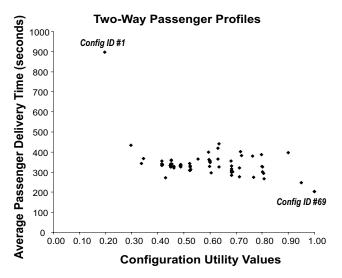
Figure 4. Average elevator performance vs. model utility for two-way traffic profiles.
