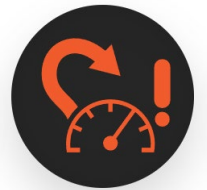
Curve Speed Warning
