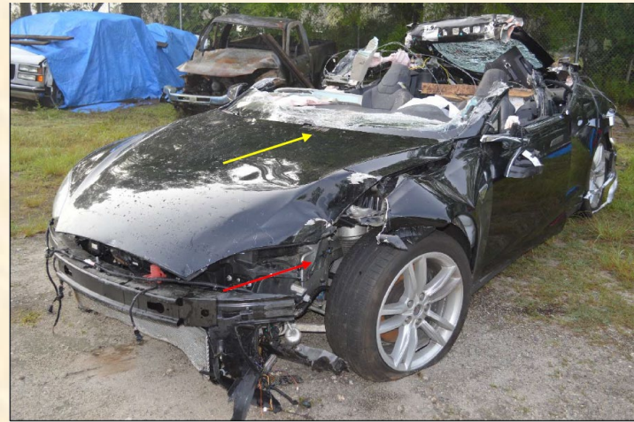
Figure 4: Florida Highway Patrol post-collision photograph depicting collision damage to Tesla. The yellow arrow indicates upper surface damage to the hood, while the red arrow indicates the pole impact damage. The rear window frame and trunk deck combination has been returned to the upright position.
