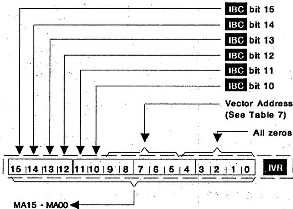
FIGURE 4. **IVR** BIT ASSIGNMENTS
