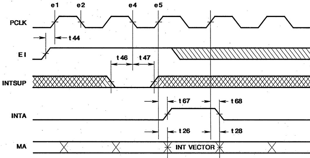
FIGURE 26. INTERRUPT TIMING: WITH NO INTERRUPT SUPPRESSION
