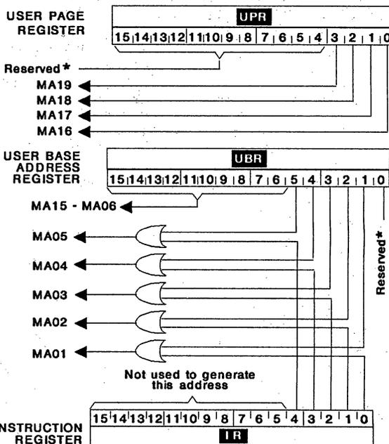
FIGURE 13. **UPR** AND **UBR** BIT ASSIGNMENTS
