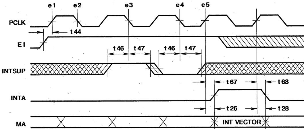
FIGURE 25. INTERRUPT TIMING: WITH INTERRUPT SUPPRESSION
