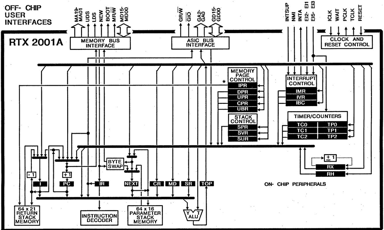
FIGURE 1. RTX 2001A FUNCTIONAL BLOCK DIAGRAM
