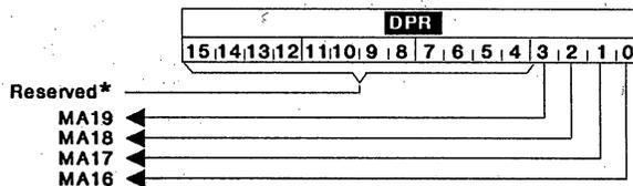
FIGURE 12. **DPR** BIT ASSIGNMENTS
